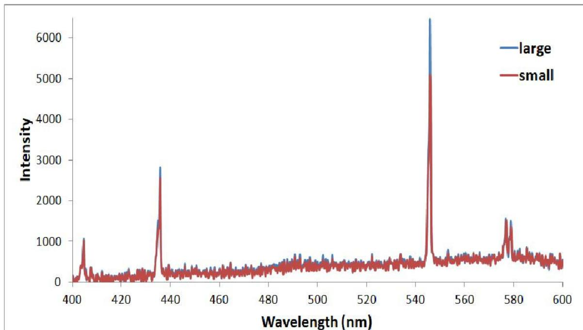
Fig. 6. The figure shows the spectrum collected between the two mirrors. The larger mirror shows larger spectrum peaks.
