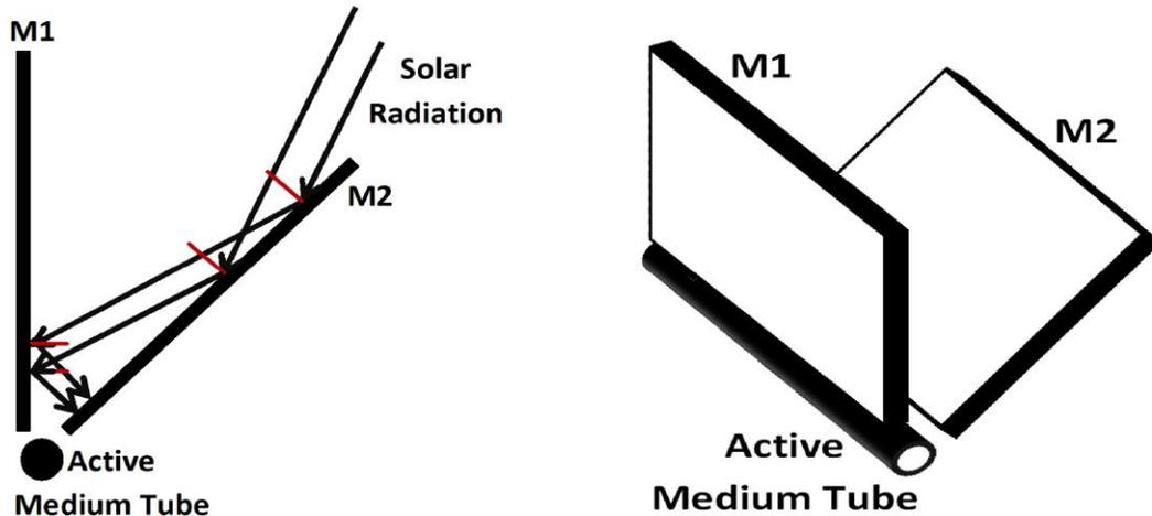
**Fig. 3.** The figure on the left shows a solar rays traces inside the concentrator. The figure on the right shows a schematic of the system used.
