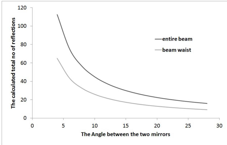
**Fig. 7.** The angle between the mirrors and the number of reflections (as an intensity indication). The entire beam curve takes in consideration all possible incidence angles. The beam waist curve considers the concentrated part of the beam that propagates about the perpendicular direction from the lamp. This curve also stimulated the behavior at the noon time where the solar radiation intensity is maximum.
