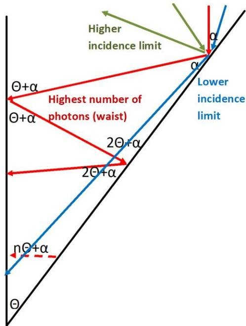
**Fig. 8.** The beam direction shown. The graph shows the parameters used in the theoretical calculations and the criteria for the beam waist calculation. The solar spectrum is considered collimated. The scanning of it throughout the day changes the direction of the beam. Although the peak exposure (the noon time) takes place at the direction indicated as the beam waist part.
