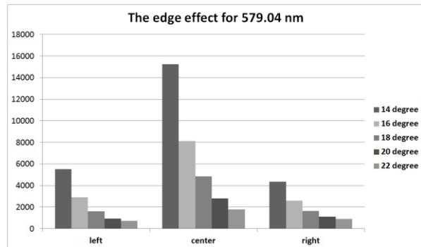
**Fig. 5.** The edge effect for different concentrator angles. It appears that the signal degradation decreases while increasing the angel between the mirrors.
