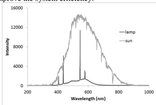
**Fig. 1.** The graph shows the spectrum for the lamp used in evaluating the design (solar simulator) against the solar spectrum (obtained outside of the lab). There are couple spectrum lines in the source spectrum. The data from those lines was compared to eliminate any cavity (resonance) effects.
