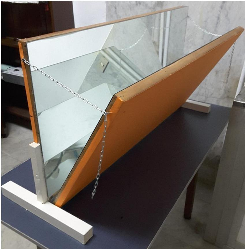
Fig. 2. A real live image of the system used. The two mirrors with the availability of changing the angle between them is shown.
