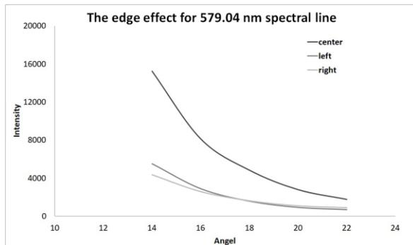
**Fig. 4.** The effect of changing the angel between the two mirrors. It appears that as the angel increases the intensity of the collected beams decreases. Increasing the angel beyond 28 degrees affects the signal drastically.
